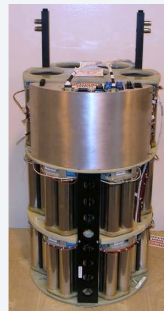
Combined 100 V and 25 V battery system for Marlin
